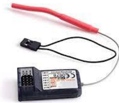
Fig. 22: Top view of FS-R6B receiver module
